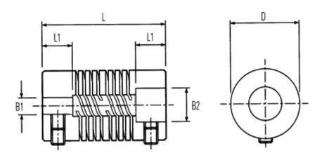
B1: Pre-drilled = 8.0B2: Pre-drilled = 12.00 D = 38.1= 66.7 L L1 = 18.0Max angular displacement = 0.60 = 22.00
